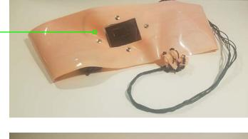
A wire connects the LCD screen in the bra, controlled via Arduino, to a set of buttons worn on teh hand.
