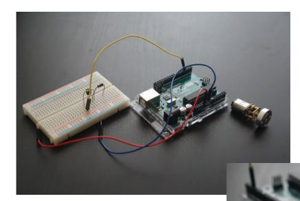
I am using an Arduino UNO to control a gear DC motor with a mount attached to it. I used Cinema 4D to model the containers, and imported the models into Autodesk Slicer to create the stacked form.
